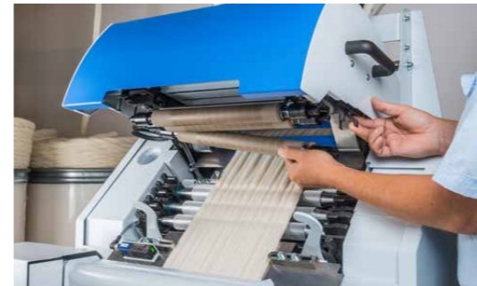
3-over-3 drafting system equipped with patented bearing solution for perfect drafting.
