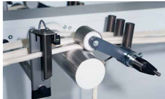
SMART CREEL with individual sliver monitoring.
