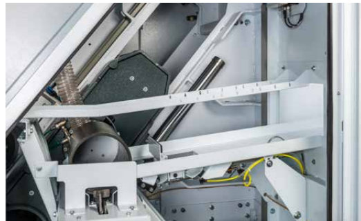
The unique lap-tube feeding device allows rapid lap changes.
