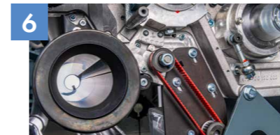
Motorized licker-in mote knife system
