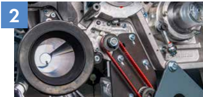
2 Motorized licker-in mote knife system PMS 2
