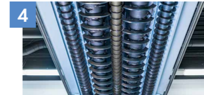
Opening rollers with high teeth density
