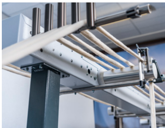
Individual sliver monitoring on SMART CREEL
