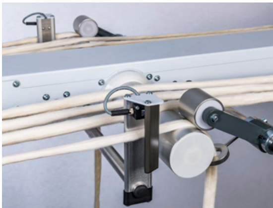
SMART sensors for individual sliver monitoring
