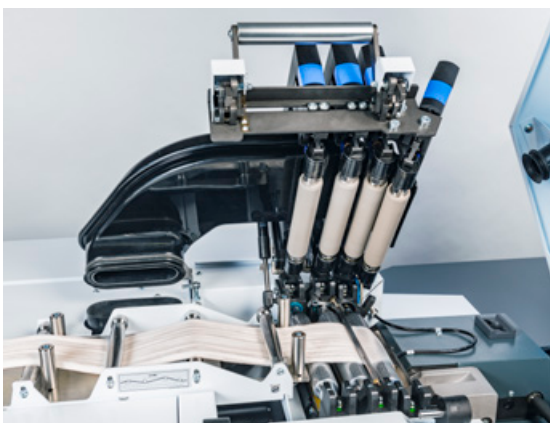
4-over-3 drafting system technology
