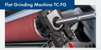
The TC-FG grinding roller grind the tips of the revolving flat by using an emery belt roller.
